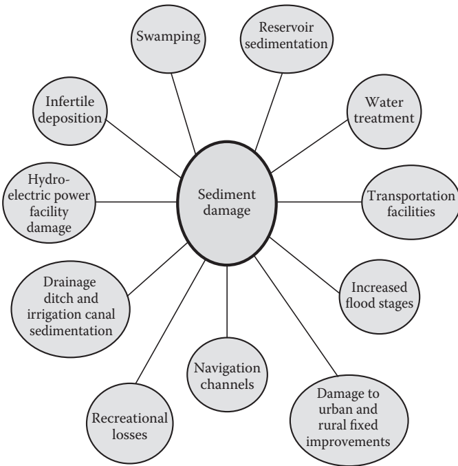
FIGURE 9.2 Types of sediment damage.
