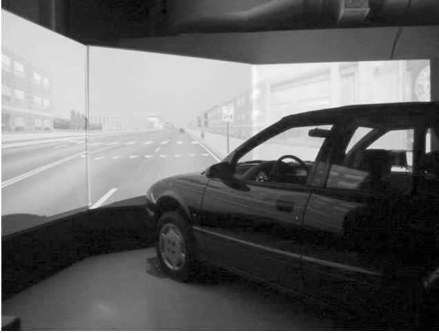
FIGURE 20.1 Driving simulator used in the route and parking choice experiments described in the text (located at the University of Massachusetts at Amherst).
